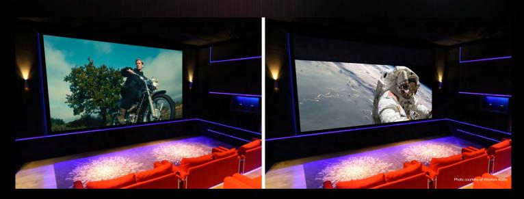
Imaging is optimum when the projected image is exactly bordered by our Infinite Black<sup>TM</sup> velvet borders, providing a significant contrast enhancement together with a real focus on the image. With the varying aspect ratios of movies, the True Aspect Masking screen masks to adjust the black borders of the image to its actual size.
