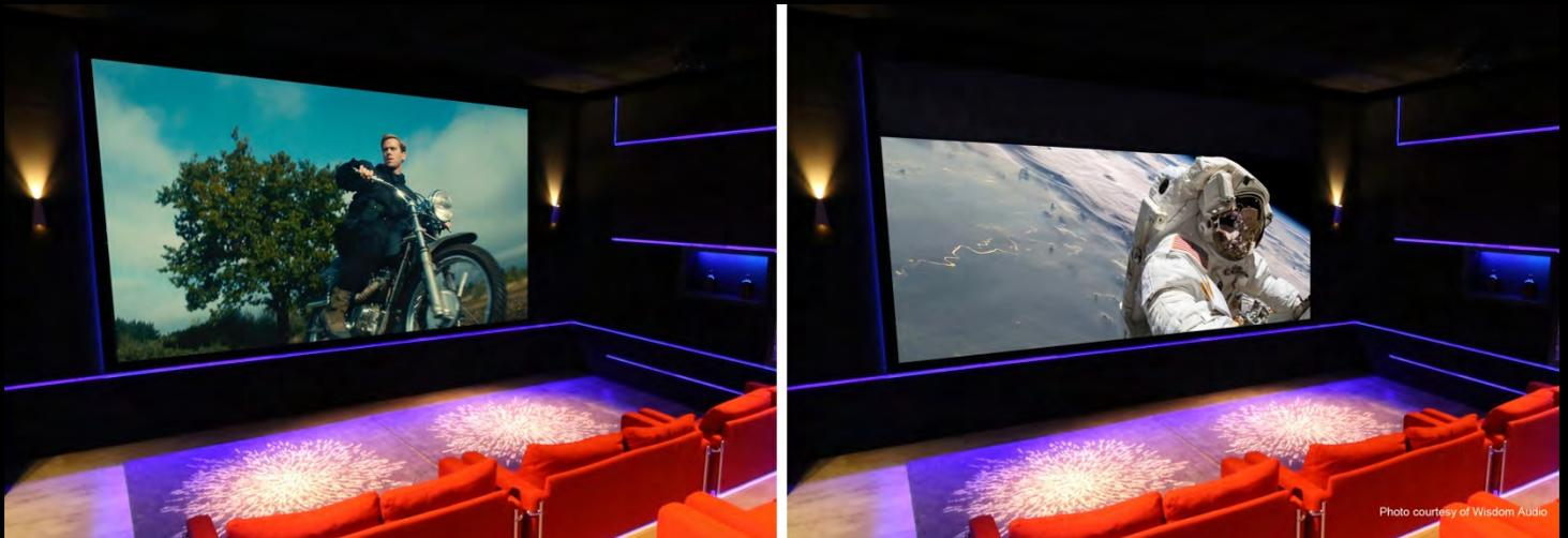
The simplest model in our mid-size masking platform, the True Aspect Masking (TAM) -1 uses one acoustically transparent mask on the top. Numerous positions such as 1.78, 1.85, 2.35, and 2.40 can be achieved through automation control.
